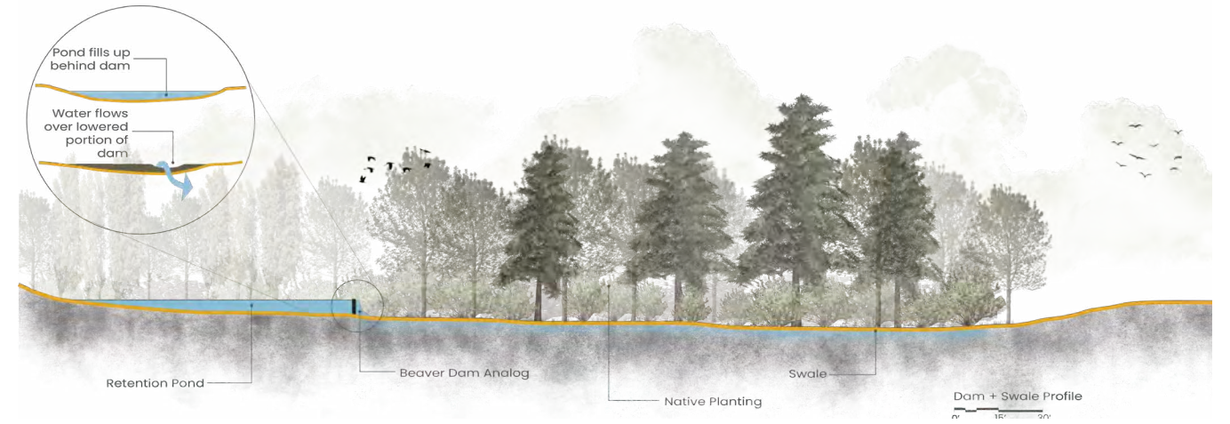
C: North-South site section through Retention Pond, Beaver Dam Analog, and Native Planting Swale. Graphic by Emma Petersen
